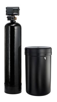
The Commercial Grade HousePure® Soft is an excellent option for larger homes and businesses that require higher flow rate and/or more water softening capacity. With 96,000 grains per gallon capacity, this 4 cubic foot softener will handle the most demanding hard water applications.
